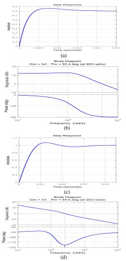
Fig. 15. Results of capacitor voltage control of AC side controller design, a. Closed-loop step response before design, b. Open-loop bode diagram before design, c. Step response after design, b. open-loop bode diagram after design
