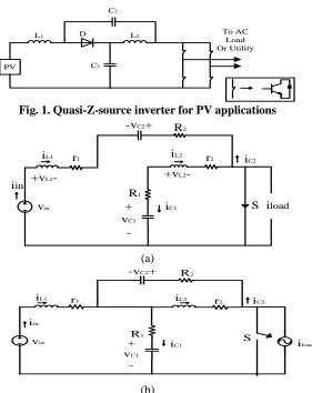
Fig. 2. The equivalent circuit for quasi-Z-source inverter equivalent: a. Shoot-through state, b. Non-shoot-through state
