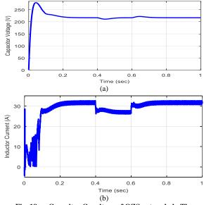
Fig. 18. a. Capacitor  $C_1$  voltage of QZS network, b. The inductance  $L_1$  current of QZS network
