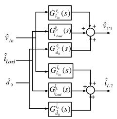
Fig. 3. Small-signal model for the quasi-Z-source network
