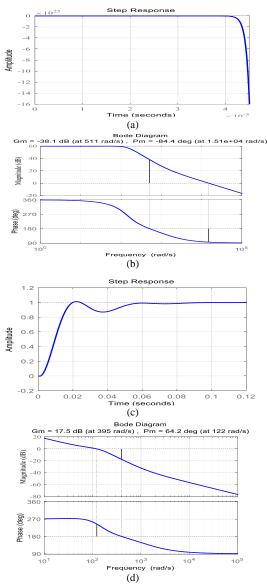
Fig. 14. Results of DC side controller design for the first method, a. Closed-loop step response before design, b. Open-loop bode diagram before design, c. Step response after design, b. open-loop bode diagram after design
