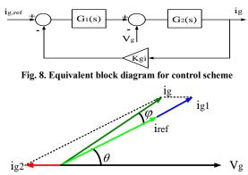
Fig. 9. Phasor diagram of grid voltage and injected current to grid  $\int_{-\infty}^{\infty} di_1$
