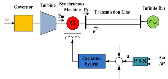
Fig. 2. Single machine infinite-bus power system
