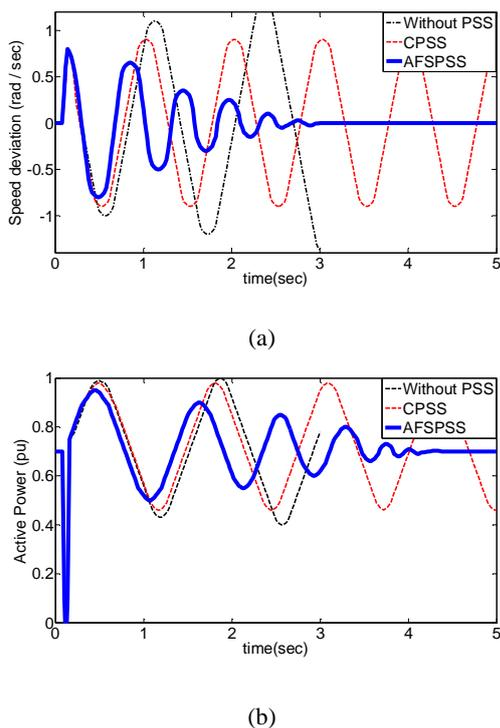
Fig. 4. Response for case 1: (a) rotor speed deviation; (b) active electrical power
