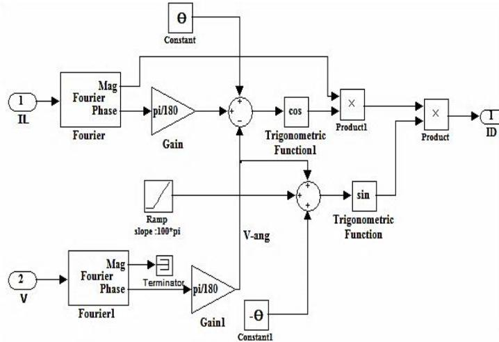
Fig. 3. Block diagram for generating  $I_D$ .
