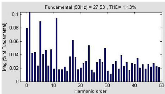
Fig. 7. Harmonic spectrum of grid current phase 'a' for NSGA-II technique.
