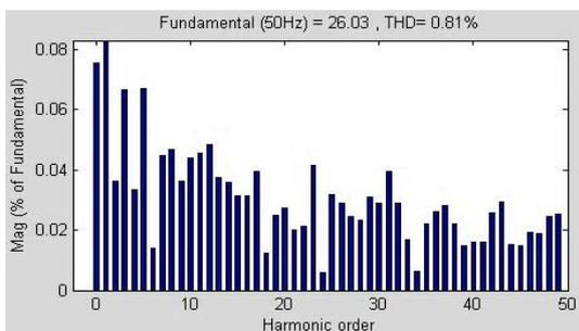
Fig. 8. Harmonic spectrum of grid current phase 'a' for SPEA2 technique.
