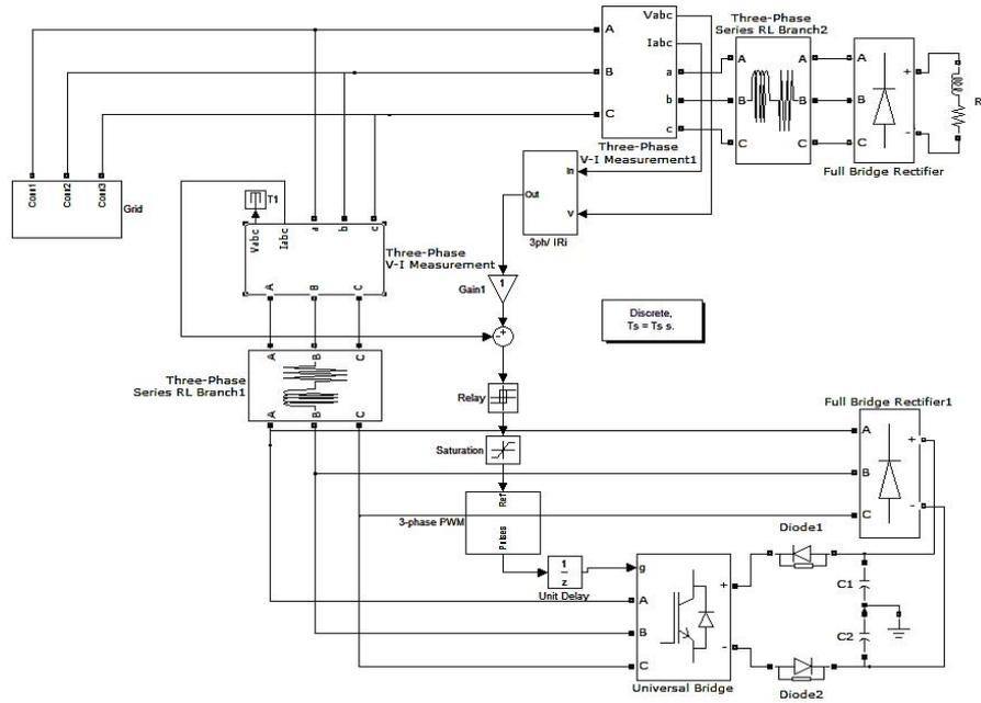
Fig. 2. The system configuration with APF.
