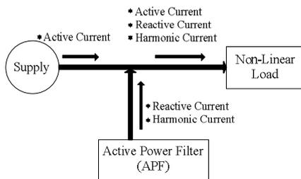
Fig. 1. Connection of shunt active filter with nonlinear load
