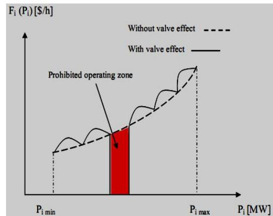
Fig. 1. Unit cost function with valve points and POZ
