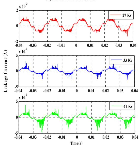
**Fig. 7.** Leakage current waveforms of insulator 1 in various voltage levels (27, 33 and 41 kV), humidity=77%, medium pollution levels.
