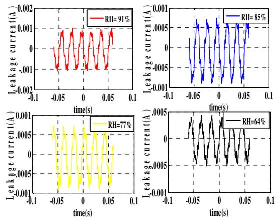
**Fig. 6.** Leakage current waveforms versus different levels of humidity (RH %) for insulator number 3.
