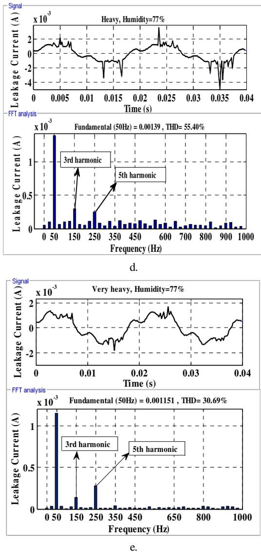
**Fig. 5.** Waveforms of the leakage current and FFT of insulator number 1 in various pollutions at 77% humidity. a. Clean, b. Light, c. Medium, d. Heavy, e. Very heavy.
