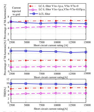
Fig. 12: Simulation results of current injected to grid for the gridconnected mode. From up: Percentage of fifth harmonic, Percentage of seventh harmonic and THD.
