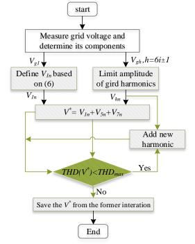
Fig. 2. Flowchart of the proposed method to generate load voltage reference for reducing harmonics of current injected to the grid.
