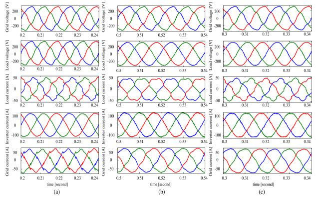
Fig. 7. Simulation results for the grid-connected mode: (a) Inverter with LCL filter (common structure), (b) Inverter with LC-L filter and with " $V_{In}$ =1p.u,  $V_{5n}$ = $V_{7n}$ =0 reference voltage", (c) Inverter with LC-L filter and with " $V_{In}$ =1p.u,  $V_{5n}$ = $V_{7n}$ =0.03p.u reference voltage". From down: grid current, inverter current, load current, load voltage, grid voltage.
