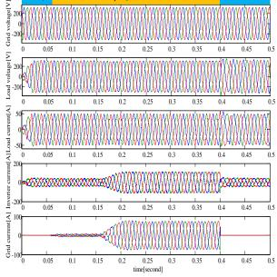
Fig. 9. Simulation results of switching between two operation modes. From down: grid current, inverter current, load current, load voltage and grid voltage.
