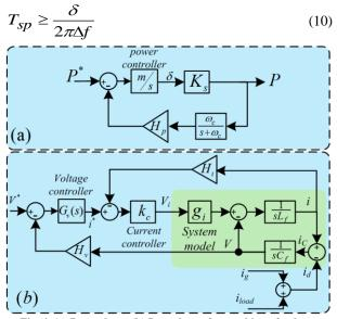
Fig. 4. (a) Power loop. (b) Inner loops for tracking of voltage reference in proposed inverter with LC-L filter in the stationary reference frame.
