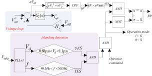
Fig. 5. Proposed logic scheme for connection to the grid and disconnection from the grid.
