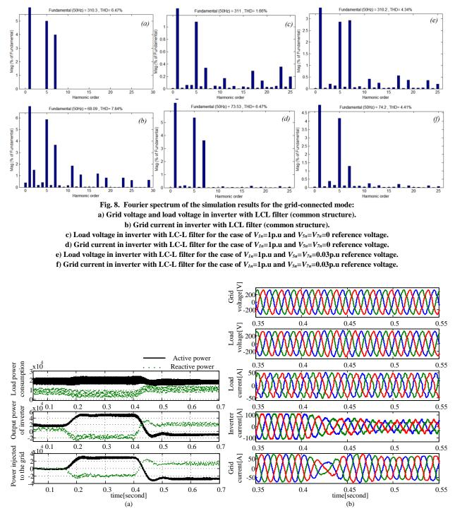
Fig. 10. Inverter with LC-L filter. A simulation results of power reference step change. (a) From down: power injected to the grid, inverter power, load power. The active and reactive power at the load, inverter and grid. (b) From down: The waveforms of the grid current, inverter current, load current, load voltage and grid voltage.
