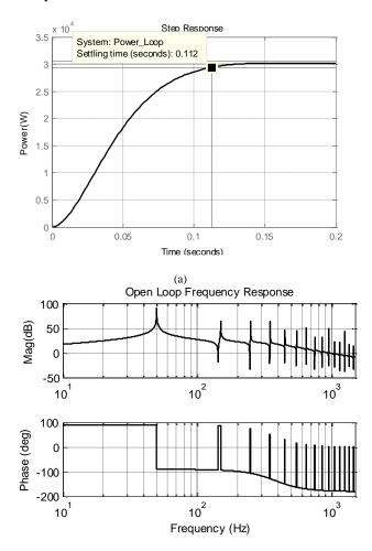
(b) Fig. 6. Inverter with LC-L filter. (a) power loop (b) open loop response for voltage loop.
