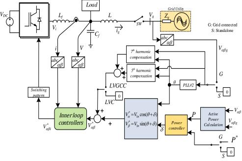
Fig. 3. Proposed inverter with LC-L filter: circuit diagram and implementation of the proposed control strategy.
