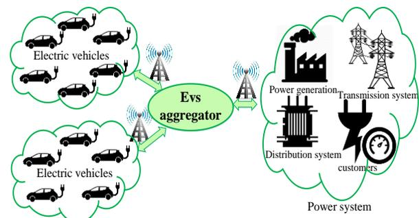
Fig. 1. The EVs aggregator as a middleman term between the power system and EVs
