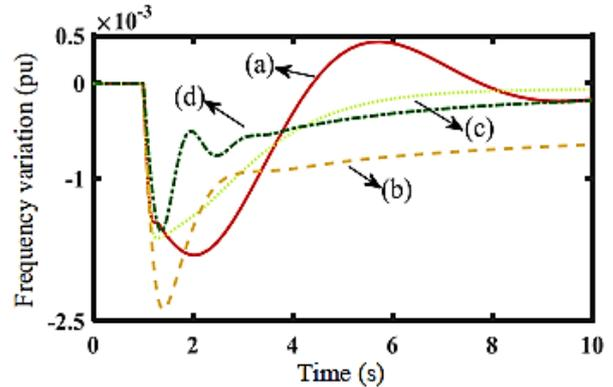
Fig. 14. Frequency variation of the LFC scheme (a) PSO-PID (b) SCA-PID (c) PSO-FOPID (d) SCA-FOPID for  $\tau(t) = e^{-2.3t}$
