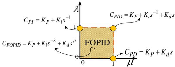
Fig. 3. The operational area of FOPID controller
