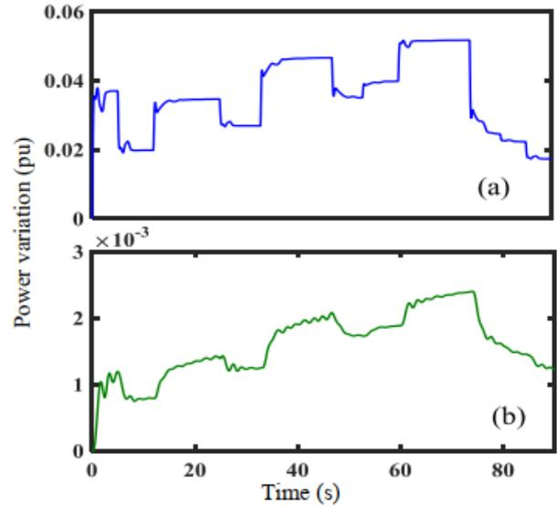
Fig. 16. Power variation of the generator (a) Area 1 (b) Area 2
