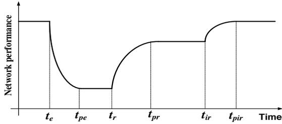
Fig. 1. The network performance associated with an extreme event [28]
