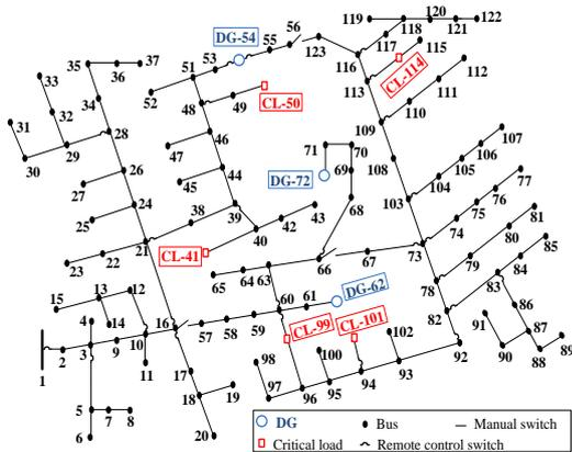
Fig. 5. Single-line diagram of IEEE 123-node distribution network
