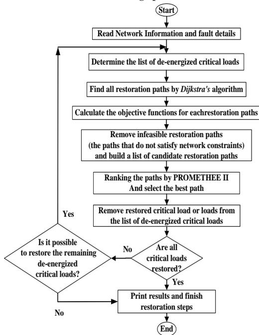
Fig. 4. The flowchart of the proposed strategy for critical load restoration
