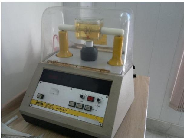
**Fig. 1. BAUR PGO S-3 device**
