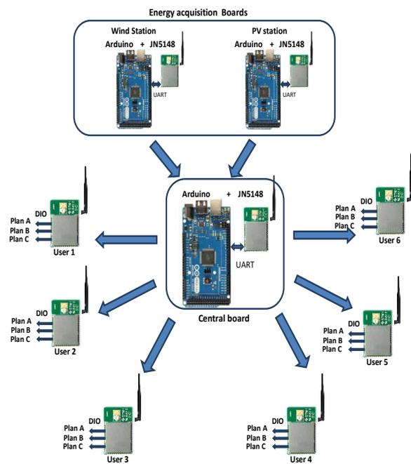
**Fig. 10. The illustration of the architecture design**
