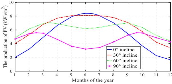
Fig. 3. The production of PV for different inclinations
