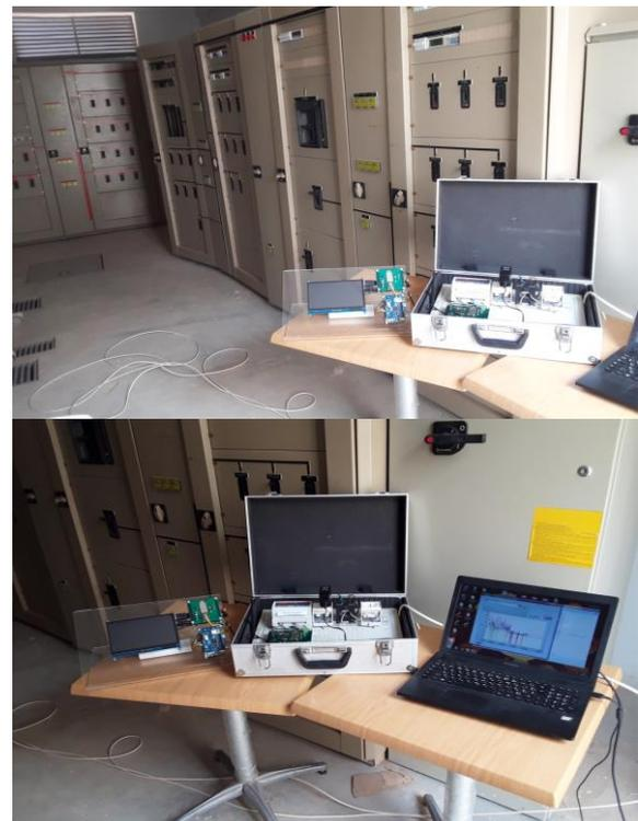
Fig.14. The prototype of the central node installed in the smart microgrid
