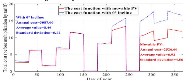
**Fig. 9. The illustration of the total annual cost of horizontal and movable PV**
