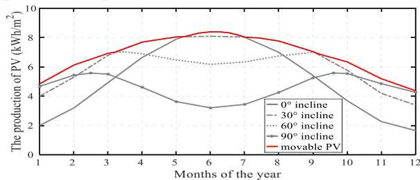
**Fig. 8. The production of a movable PV**
