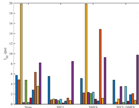
Fig. 18. The maximum fault current of the transmission lines in scenario 1
