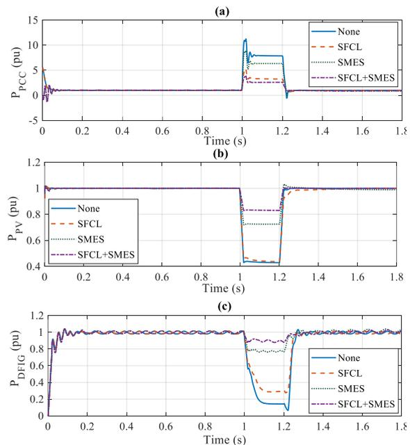
**Fig. 15. Diagram of (a) P<sub>PCC</sub> (b) P<sub>PV</sub> (c) P<sub>DFIG</sub> in the scenario 1**
