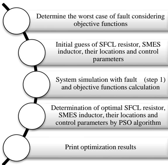
Fig. 8. the algorithm of SMES and SFCL allocation in single-step optimization
