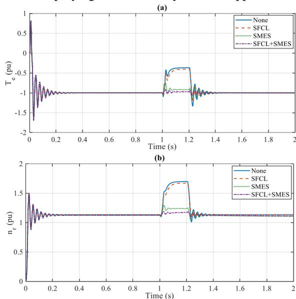
Fig. 16. The diagrams of (a) electromagnetic torque (b) rotor speed of DFIG in scenario 1
