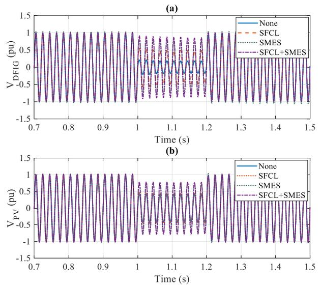
**Fig. 14. Output voltage diagram of (a) DFIG (b) PV in scenario 1**
