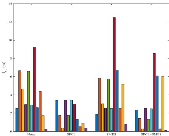
Fig. 22. The maximum fault current of the transmission lines in scenario 2
