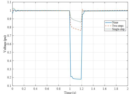
**Fig. 11. The DFIG bus Voltage**
