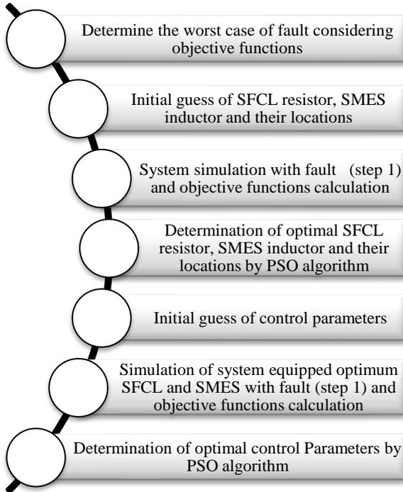
Fig. 7. the algorithm of SMES and SFCL allocation in two-step optimization
