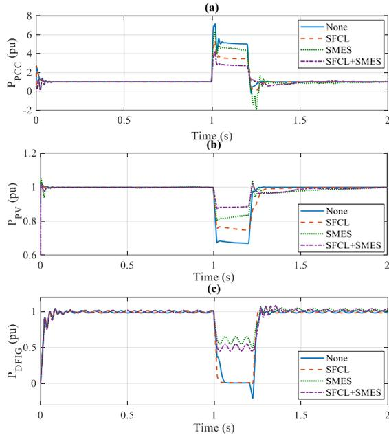
Fig. 20. Diagram of (a)  $P_{PCC}$  (b)  $P_{PV}$  (c)  $P_{DFIG}$  in scenario 2
