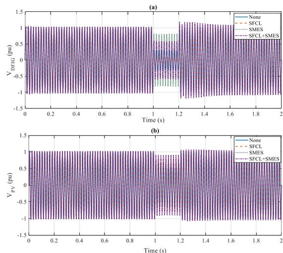
Fig. 19. Output voltage diagram of (a) DFIG (b) PV in scenario 2
