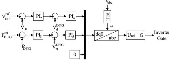
Fig. 6. The control diagram of the SMES inverter
