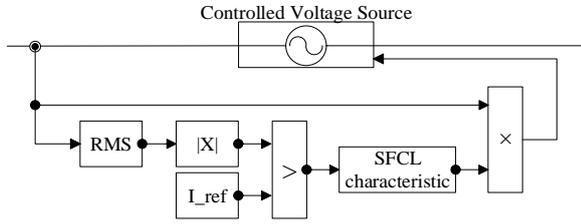
Fig. 3. The control diagram of the SFCL
