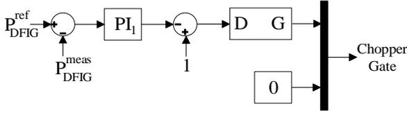
Fig. 5. The control diagram of the chopper
