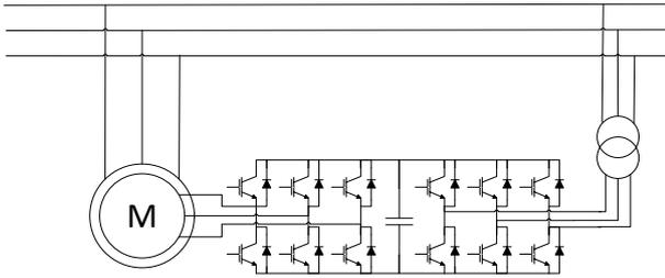
Fig. 1. The grid connection of the wind turbine
