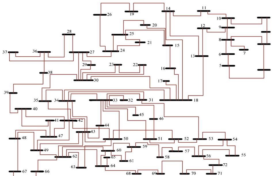
Fig. 2. Single-line diagram of network 400 kV in Iran
