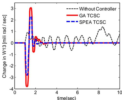
**Fig. 8.** Response of  $\Delta\omega_{13}$  for light load condition
