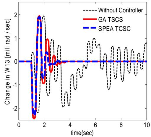
Fig. 14. Response of  $\Delta\omega_{13}$  for heavy load condition
