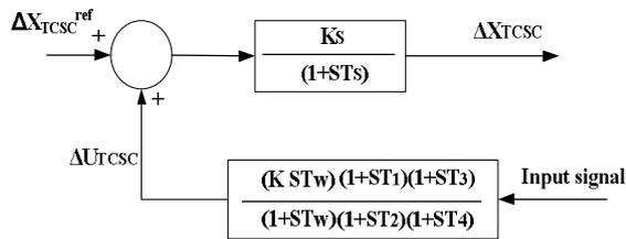
Fig. 2. Block diagram of TCSC
