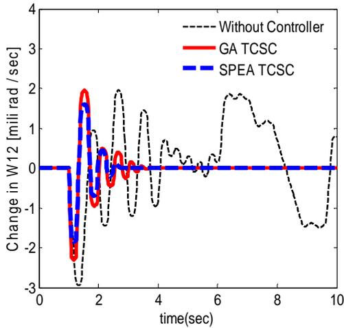
Fig. 12. Response of  $\Delta\omega_{12}$  for heavy load condition
