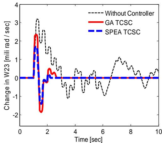
**Fig. 7.** Response of  $\Delta\omega_{23}$  for light load condition
