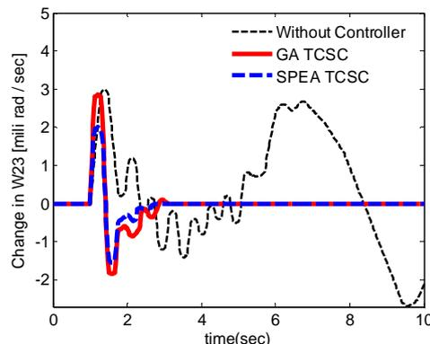
**Fig. 10.** Response of  $\Delta\omega_{23}$  for normal load condition
