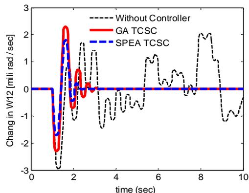
**Fig. 9.** Response of  $\Delta\omega_{12}$  for normal load condition
