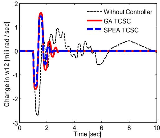
**Fig. 6.** Response of  $\Delta\omega_{12}$  for light load condition
