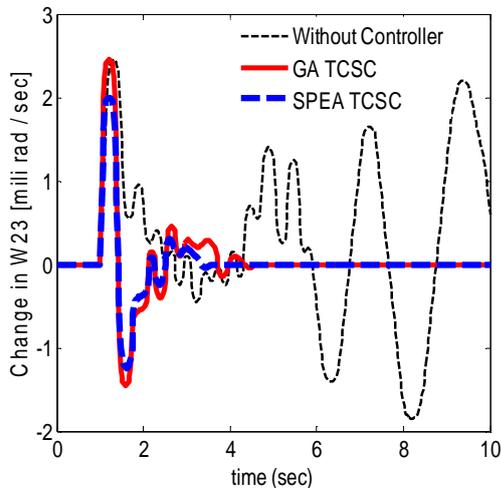
Fig. 13. Response of  $\Delta\omega_{23}$  for heavy load condition
