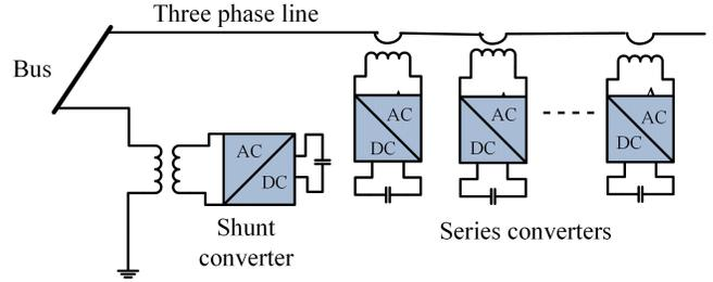
Fig. 1. Block diagram of DPFC [27]
