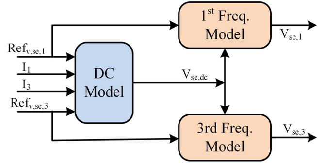
Fig. 2. Series converter modeling
