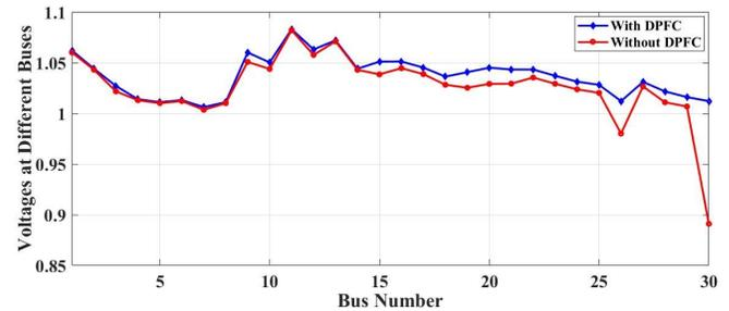
Fig. 9. Bus Voltage magnitude (in p.u.) of IEEE-30 bus system
