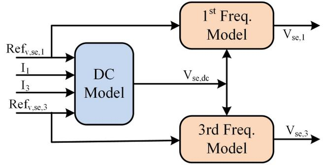
Fig. 2. Series converter modeling
