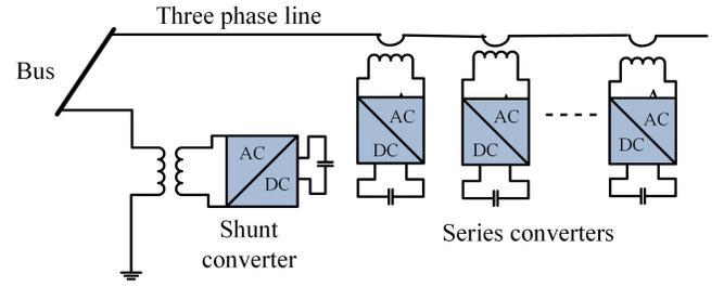
Fig. 1. Block diagram of DPFC [27]
