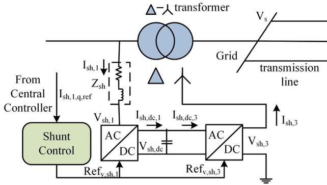
Fig. 3. Shunt converter modeling
