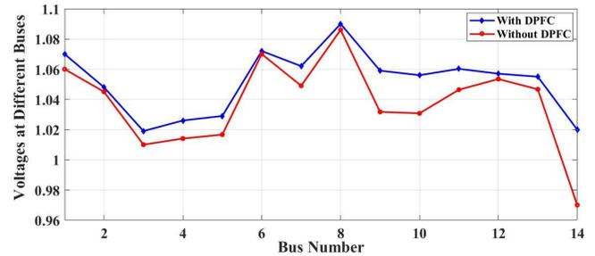
Fig. 7. Bus voltage magnitude (in p.u.) of IEEE-14 bus structure
