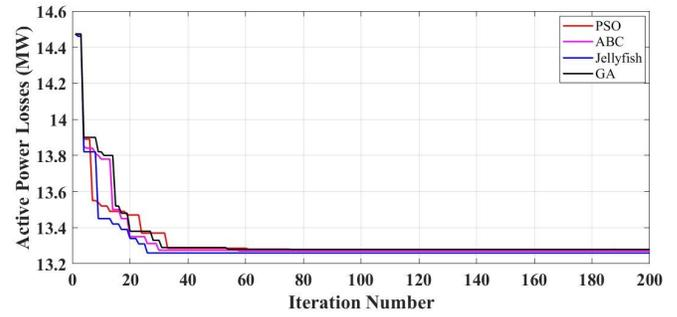
Fig. 6. Convergence graph of PSO, ABC, and jellyfish optimization for IEEE-14 bus structure
