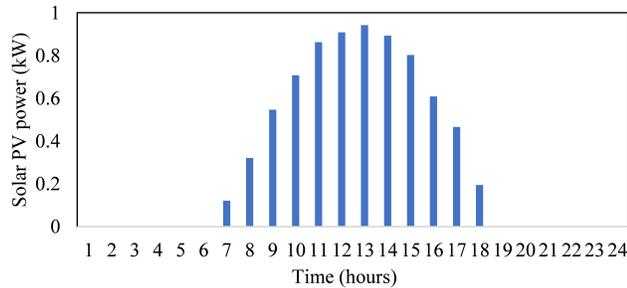
Fig. 3. Solar power generated by PV panels
