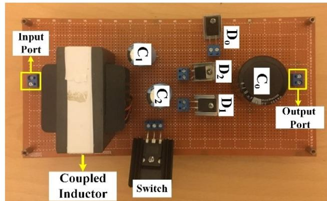
Fig. 9. Experimental prototype of the suggested converter
