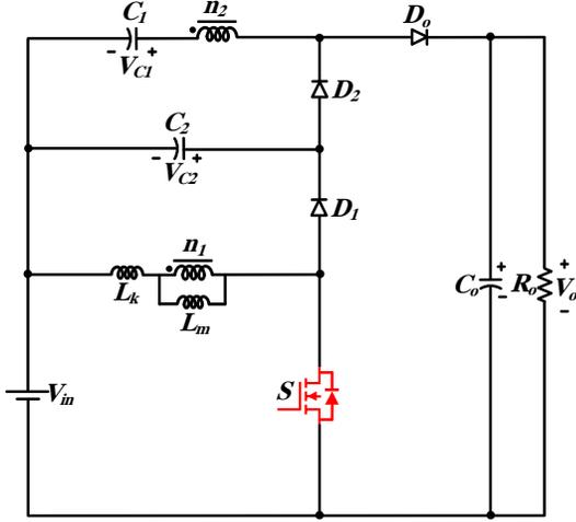
Fig. 1. Configuration of the suggested coupled inductor-based topology.
