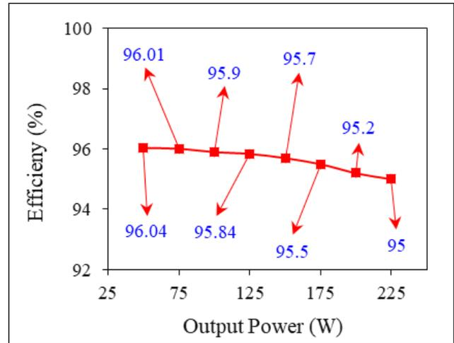
Fig. 8. The measured efficiency curve versus output power
