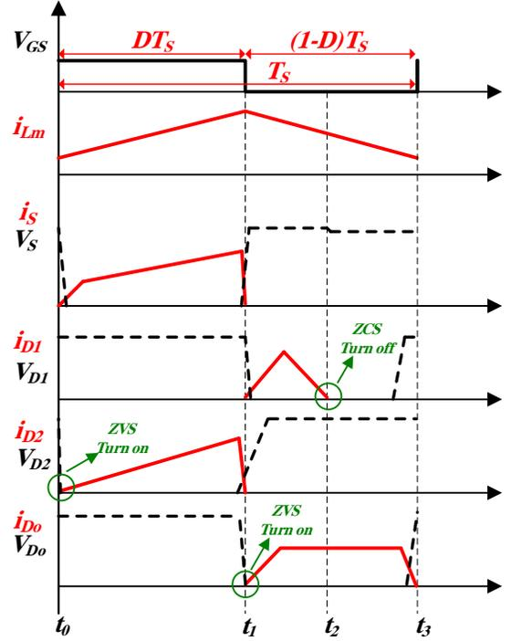
Fig. 2. Time waveform of the suggested converter.
