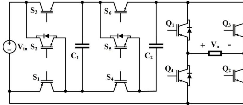
Fig. 1. Configuration of proposed 7-level switched-capacitor inverter
