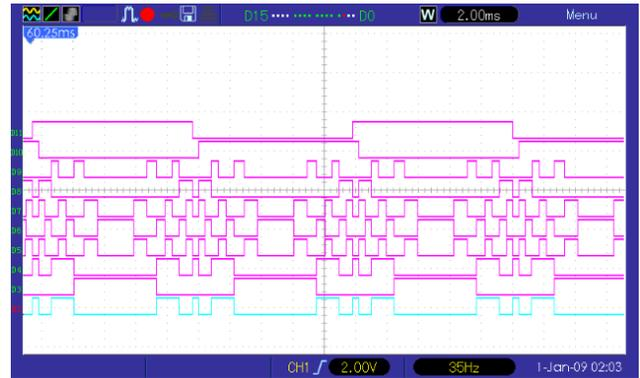
Fig. 11. Experimental test results; generated gate pulses for 17-Level inverter switches
