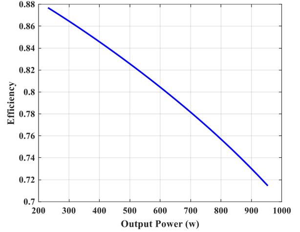
Fig. 4. Efficiency of proposed seven-level inverter
