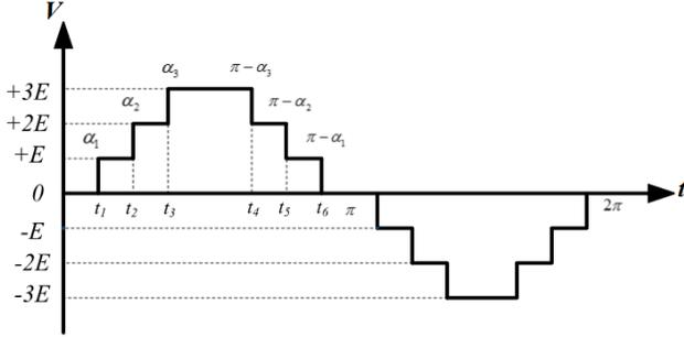
Fig. 3. Staircase modulation
