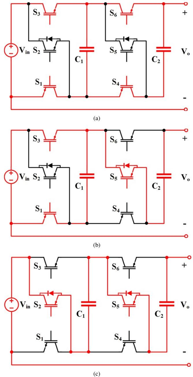
Fig. 2. Operating modes of the suggested switched-capacitor unit; (a) Mode 1, (b) Mode 2, (c) Mode 3
