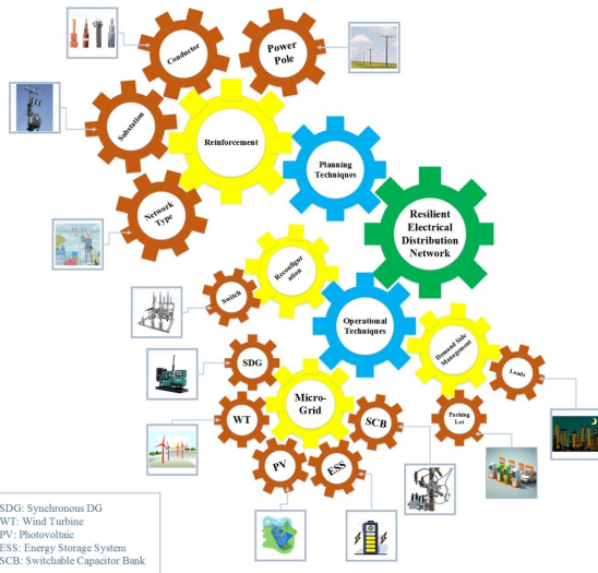
Fig. 1. Classification of resiliency improvement techniques of electrical distribution network.
