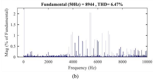
Fig. 8. Output voltage in OVHC mode of the proposed method: a) waveform b) harmonic spectra
