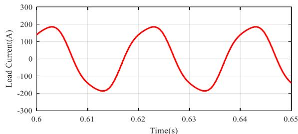
Fig. 17. Load current in CCHC mode of the proposed method
