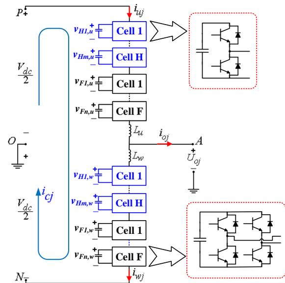
Fig 1. One leg structure of Hybrid-MMC
