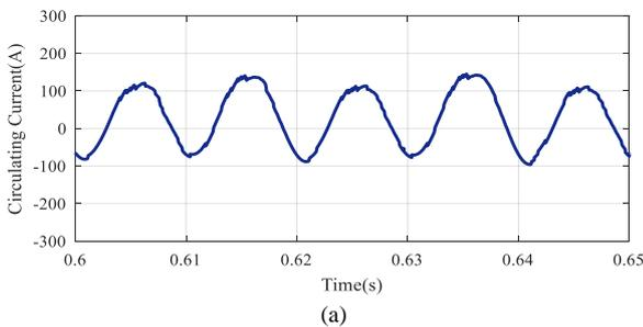
Fig 7. Circulating current in CCHC mode of the traditional method: a) waveform b) harmonic spectra
