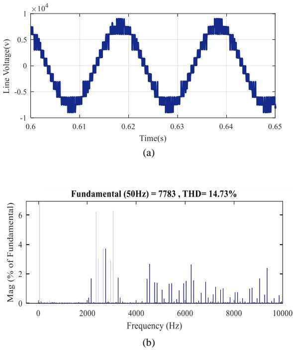
Fig 6. Output voltage in CCHC mode of the traditional method: a) waveform b) harmonic spectra
