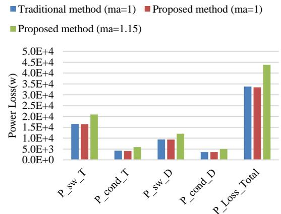
Fig. 19. Hybrid-MMC losses in CCHC mode
