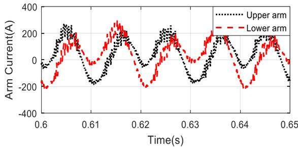
Fig. 11. Arm currents in OVHC mode of the proposed method
