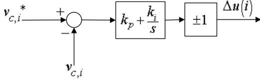
Fig 2. Block diagram of the capacitors' voltage control method
