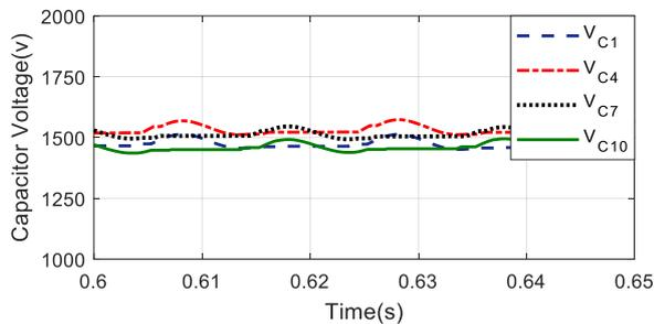
Fig. 15. Capacitor voltages of SMs in CCHC mode of the proposed method
