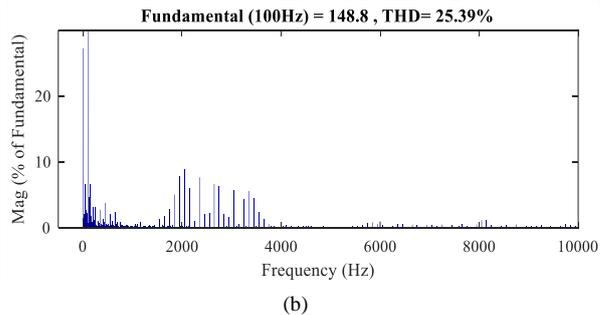
Fig. 9. Circulating current in OVHC mode of the proposed method: a) waveform b) harmonic spectra
