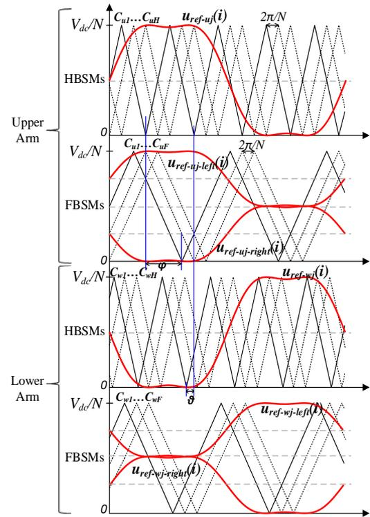
Fig 3. Modulation waveforms
