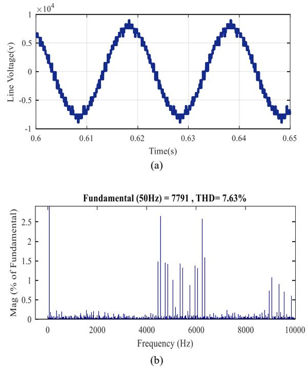
**Fig 4.** Output voltage in OVHC mode of the traditional method: a) waveform b) harmonic spectra
