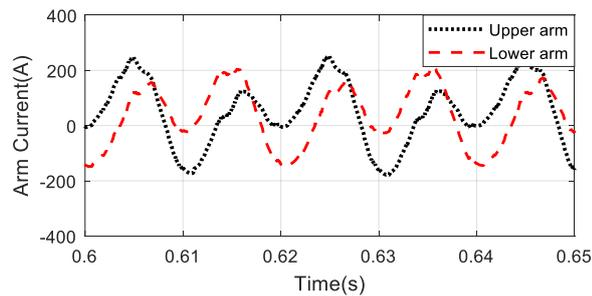
Fig. 16. Arm currents in CCHC mode of the proposed method
