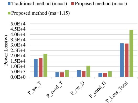
Fig. 18. Hybrid-MMC losses in OVHC mode
