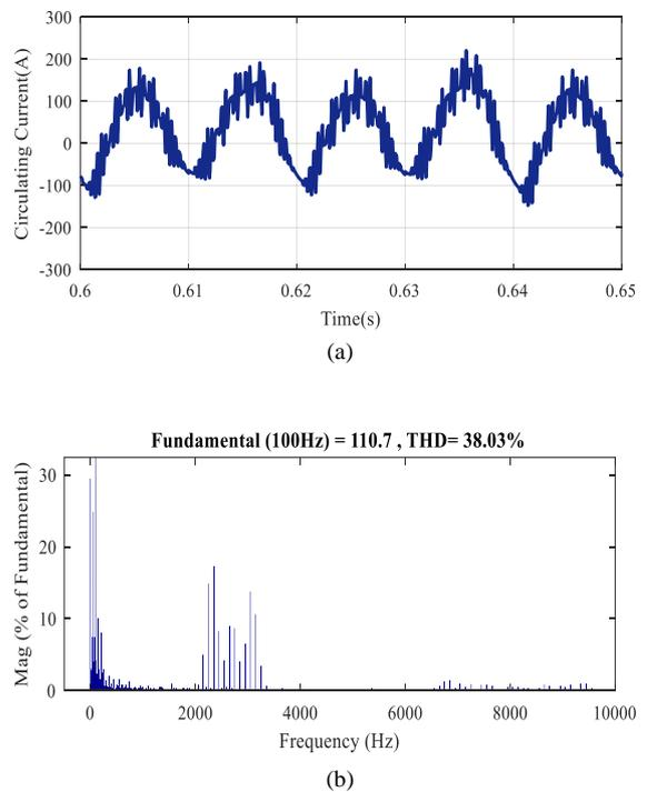
**Fig 5.** Circulating current in OVHC mode of the traditional method: a) waveform b) harmonic spectra
