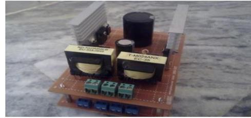
Fig. 26. Experimental prototype of the proposed converter.
