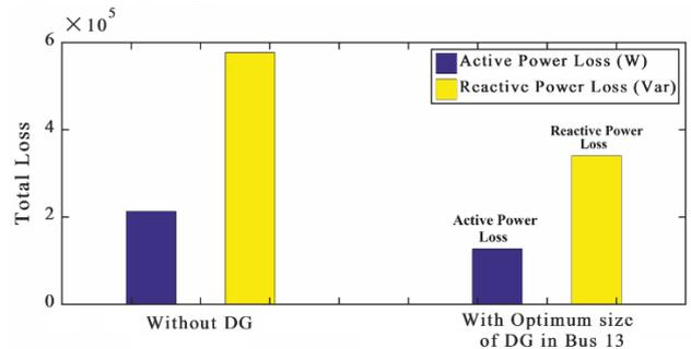
Fig. 8. System power losses with / without optimal DG
