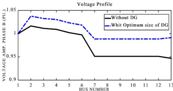
Fig. 9. Voltage profile of phase B with / without DG optimum size
