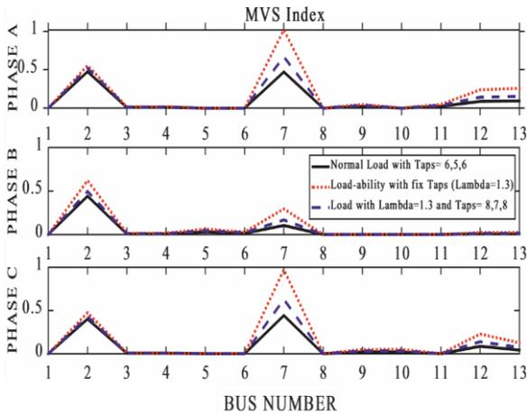
Fig. 7. Three-phase voltage stability index for maximum load-ability
