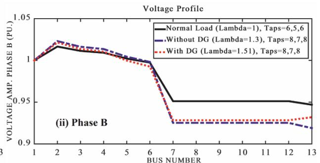
Fig. 10. The load-ability effect on the voltage profile (i) phase A, and (ii) phase B; with / without DG
