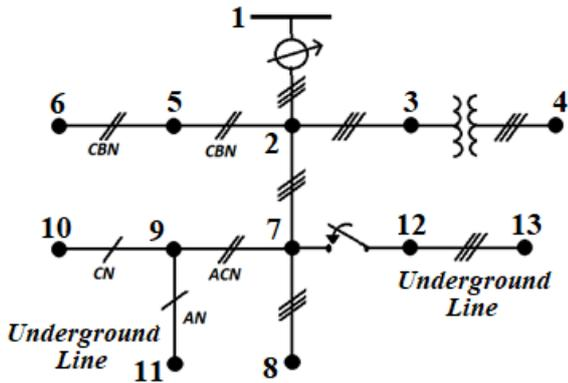
Fig. 5. IEEE13bus distribution test system
