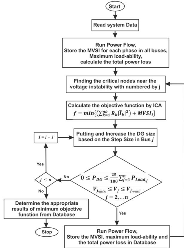
Fig. 4. Optimization schedule flowchart for allocation and size of DG
