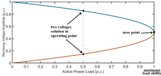
Fig. 3. Two voltage solutions and PV curve.
