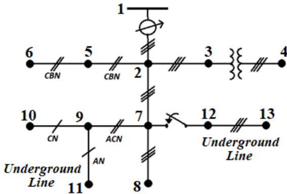
Fig. 5. IEEE13bus distribution test system
