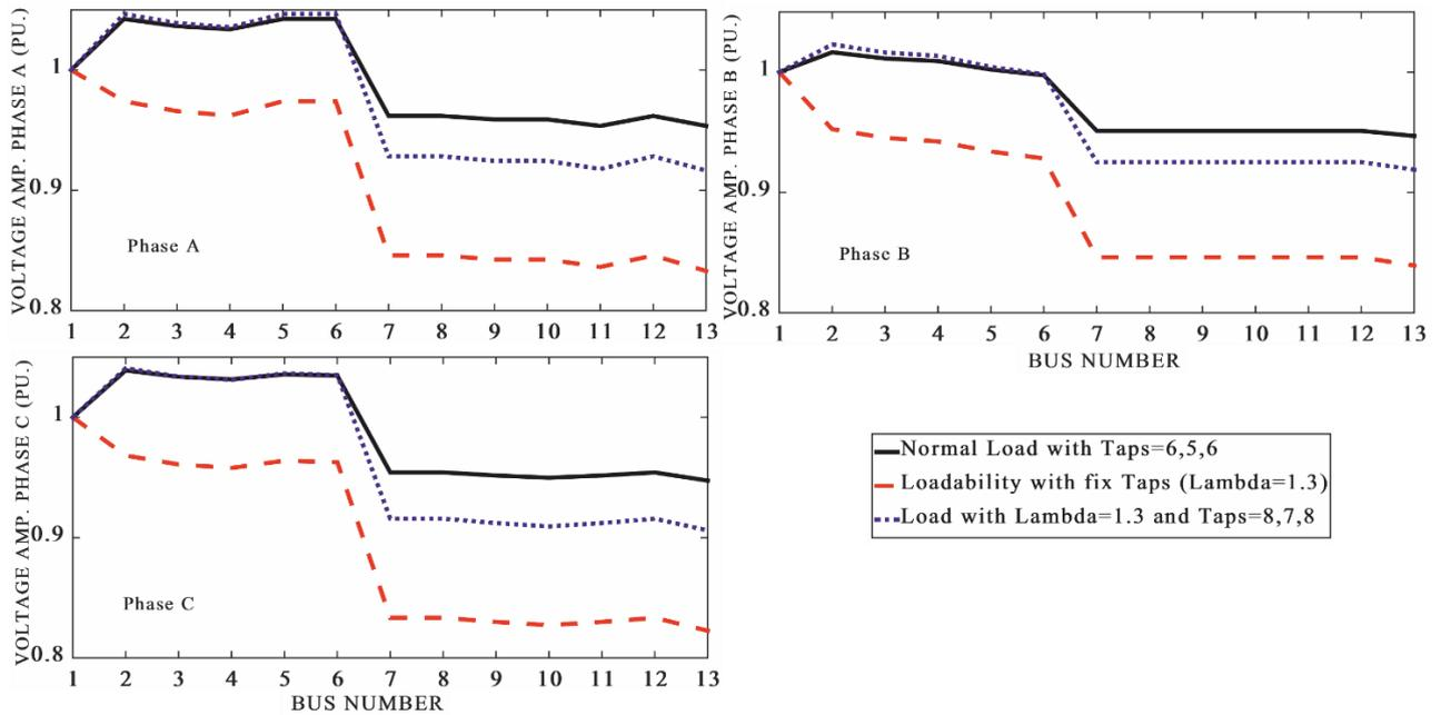
Fig. 6. voltage profiles of three phase for maximum load-ability; i) Phase A , ii) Phase B , iii) Phase C
