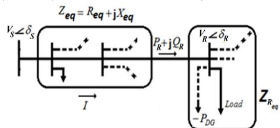
Fig. 2. Equivalent circuit seen from each bus of the DEN
