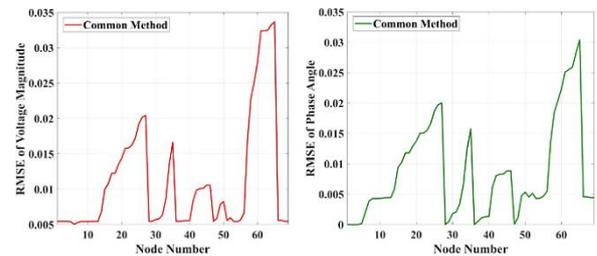
Fig.7. RMSE values for voltage amplitude and phase angle for all nodes of the network in the common method.
