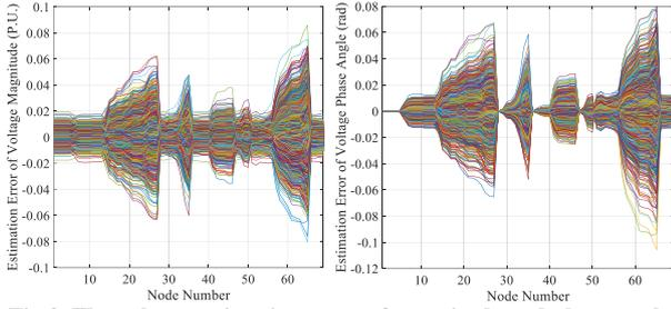
**Fig.9. The voltage estimation error of magnitude and phase angle in the common method.**
