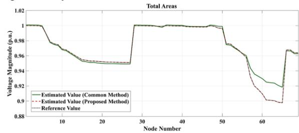
Fig.6. Voltage amplitude state estimation values of the proposed method and the common method.
