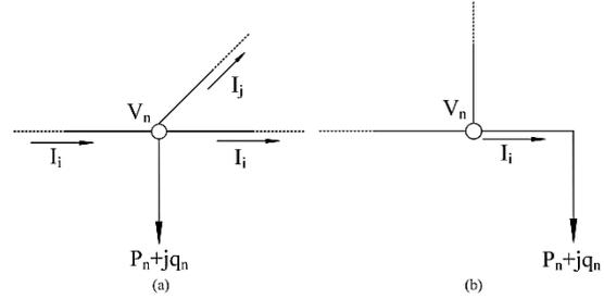
Fig.1. (a) The load connected to the branching node. (b) The load connected to the feeder end node.
