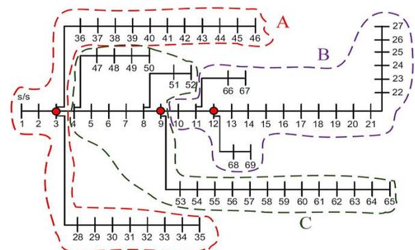
Fig.3. Dividing the IEEE 69-bus network into multiple sub-areas
