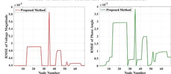
Fig.8. RMSE values for voltage amplitude and phase angle in all nodes of the network in the proposed method.
