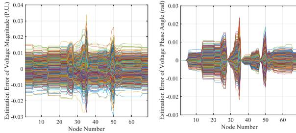
**Fig.10. The voltage estimation error of magnitude and phase angle in the proposed method.**
