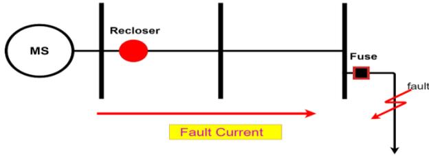
Fig. 2. Radial distribution networks no dg
