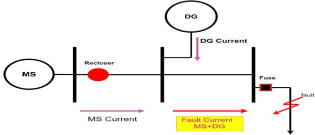
Fig. 3. Radial distribution networks with DG
