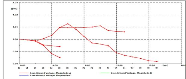
buses voltage profile after installation DGs
