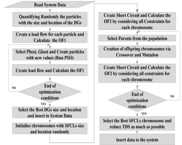
**Fig. 5. The Flowchart of the proposed design**
