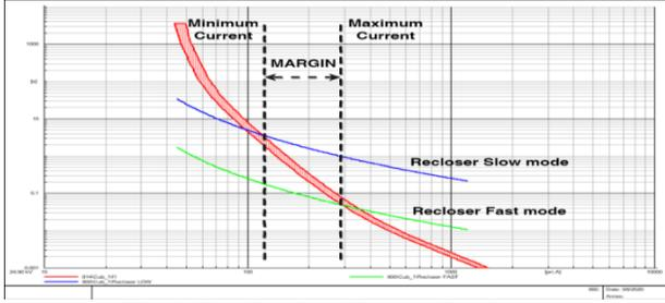
Fig. 1. Coordination of fuses and reclosers
