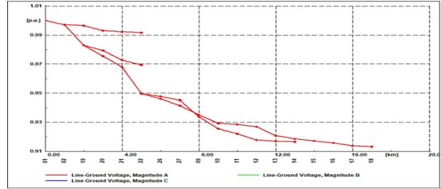
buses voltage profile before installation DGs
