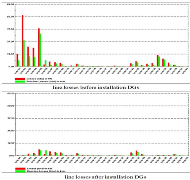
Fig. 9. All line energy losses before and after installation DGs
