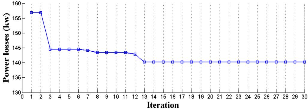
(a). Power losses vs. iteration.
