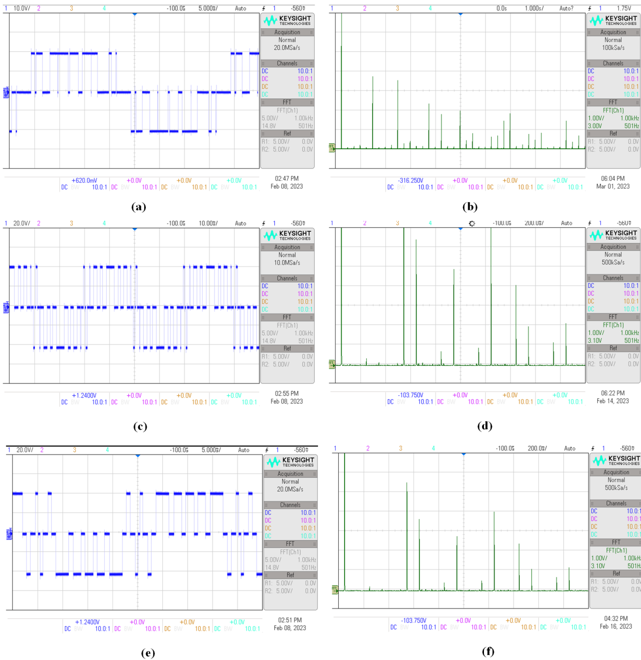
Fig. 5. Sensed Waveforms in DSO (a) S - PWM Voltage (b) FFT of S - PWM Voltage (c) SHE - PWM Voltage (d) FFT of SHE - PWM Voltage (e) P - PWM Voltage (f) FFT of P - PWM Voltage.
