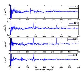
Fig. 7. Radial vibration signals at constant load condition: (H) Healthy, (IR) Inter race, (OR) Outer race, (BB) Ball broken conditions.
