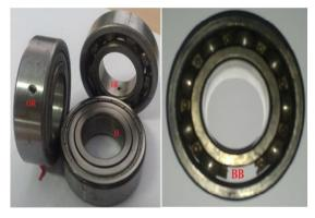
Fig. 4. Healthy bearing (H), Outer race fault(OR), Inner race fault(IR), Ball broken fault bearing(BB).
