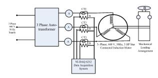
Fig. 2. Schematic diagram of the proposed scheme.
