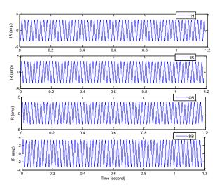
Fig. 6. Current signal at constant load condition: (H) Healthy, (IR) Interrace, (OR) Outer race, (BB) Ball broken conditions.
