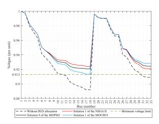
Fig. 8. Voltage profiles of the 33-bus distribution network.
