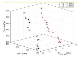
Fig. 9. The pareto front solutions obtained with 75% and 95% confidence intervals of the power losses using the MOPSO algorithm.
