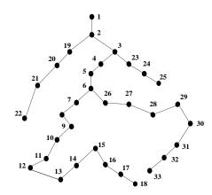
Fig. 4. The IEEE 33-bus test distribution network diagram.
