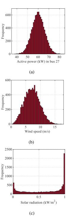
Fig. 5. The corresponding histograms of the demand load at bus 27, wind speed, and solar radiation samples.
