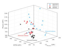
Fig. 11. The obtained Pareto front solutions of the 118-bus distribution network using MOPSO, NSGA II, and MOGWO algorithms.
