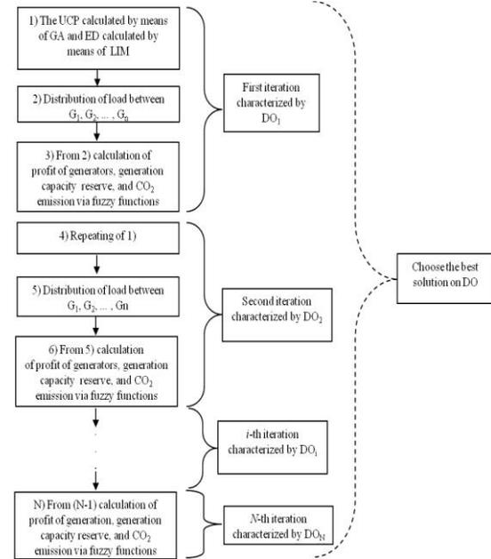
Fig. 4. The degree-of-optimality based algorithm (the algorithm designed to find the largest DO<sup>system</sup>).
