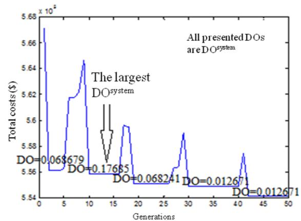
Fig. 8. The  $DO_{system}$  for three considered system's attributes, and for the fifth hour of a 24-hour time period (the analogous diagrams for the 23 other one-hour periods of a 24-hour time duration are not shown).
