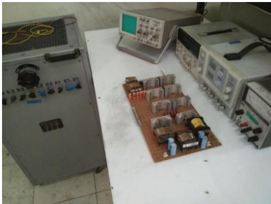
Fig. 8. The experimental prototype of the proposed converter.
